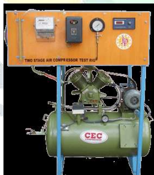
Figure 2.1 Test rig of Two stage reciprocating Air compressor.
