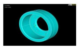
A brake drum assembly of a light passenger vehicle which is used for the analysis is shown in Figure 3.1. The drum brake consists of backing plate, brake shoes, brake drum, wheel cylinder, return springs and a self adjusting system. Brake shoes consist of a steel shoe with the friction material lining riveted or bonded to it.
