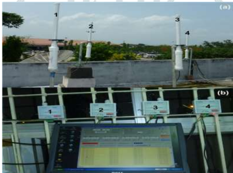
Fig. 3: Calibration and Validation of Lightning sensors at RMC, Guwahati. Network of 4-lightning sensors and (b)4-Data acquisition systems. 4 th lightning sensor cables are connected to Note Book Computer for collecting data from the Sensor .
