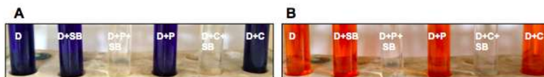
Figure 7. Complete decolorization of (A) trypan blue, and (B) congo red with sodium borohydride in presence of SNP. Abbreviations: D (dye); SB (sodium borohydride); P (PSNPs); C (CSNPs).
