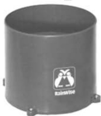
Fig.1 Rainwise tipping bucket
