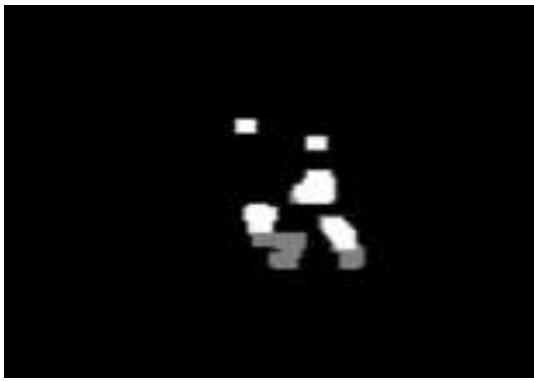
Figure 12 Opening result of MOG
