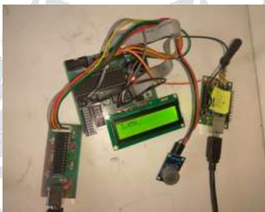
Fig 2. Testing of MQ7 sensor
