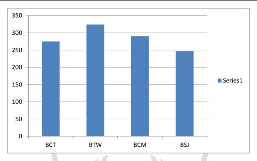
The fabric of bamboo from the four structures in the test of the air permeability. So it is conclude that Air permeability of bamboo Twill weave gives good result compared to single jersey, cross miss, cross tuck.
