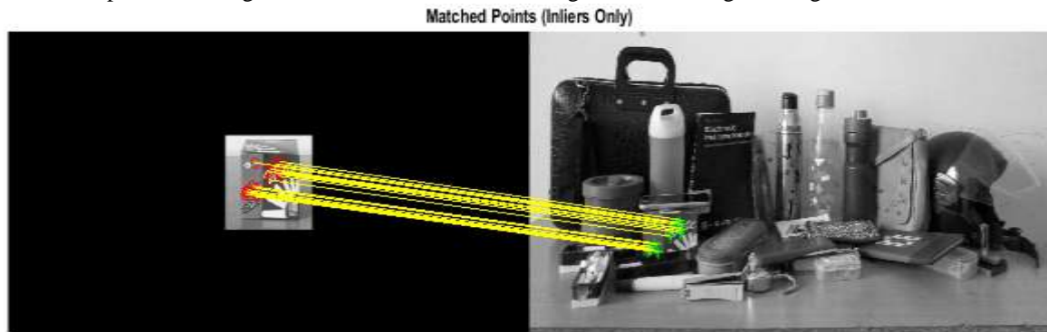
Fig. 5 Matching of Chalk Box with Cluttered image by removing outliers (SURF Method)
