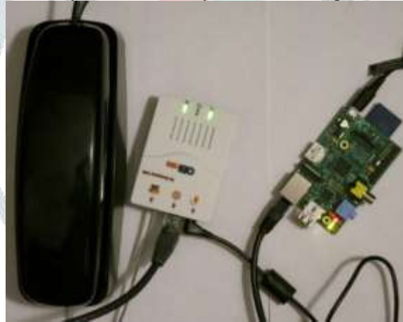
Figure 3: Landline using RPi and Google Voice
