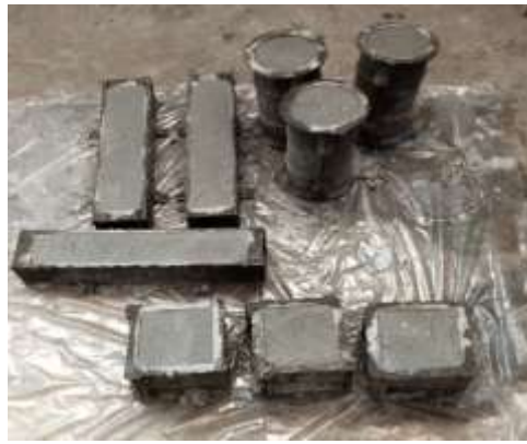
Figure 5: Shows Casted specimens before de-moulding
