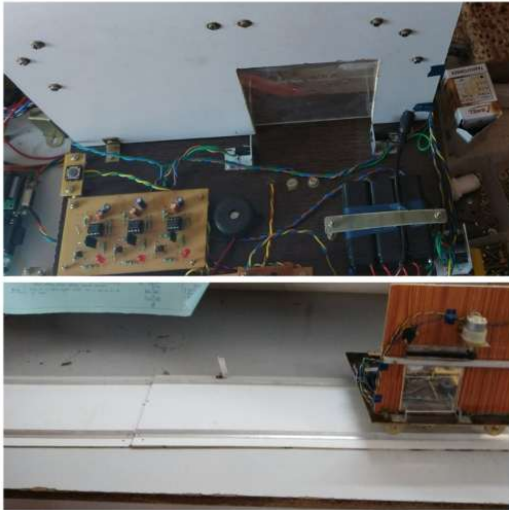
Fig 9 : Final Prototye design of Driverless Shuttling Train
