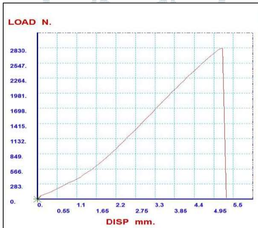
Figure 16: Banana tensile test graph
