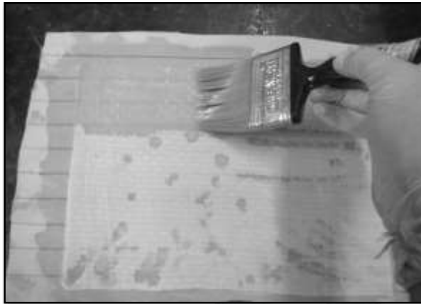
Figure 2: Hand molding process (Applying resin)
