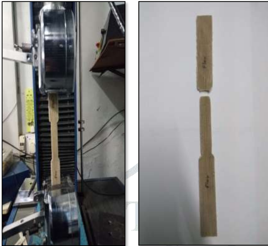
Figure 19: Tensile test of flax specimen
