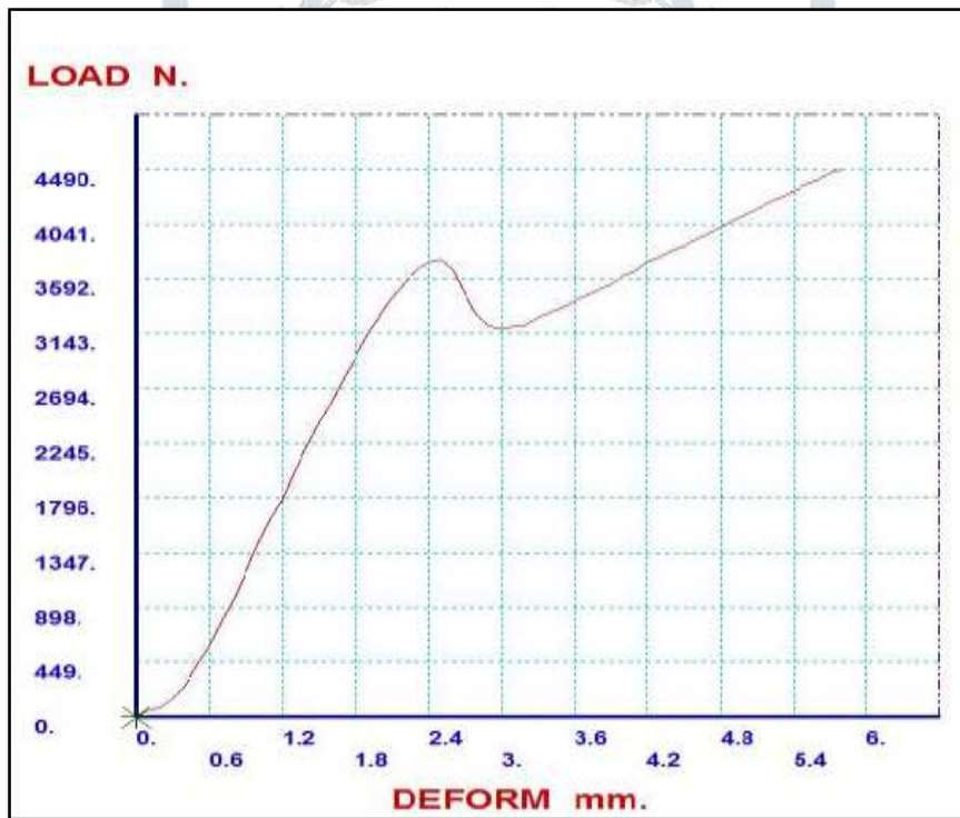
Figure 21: Compression test of flax specimen
