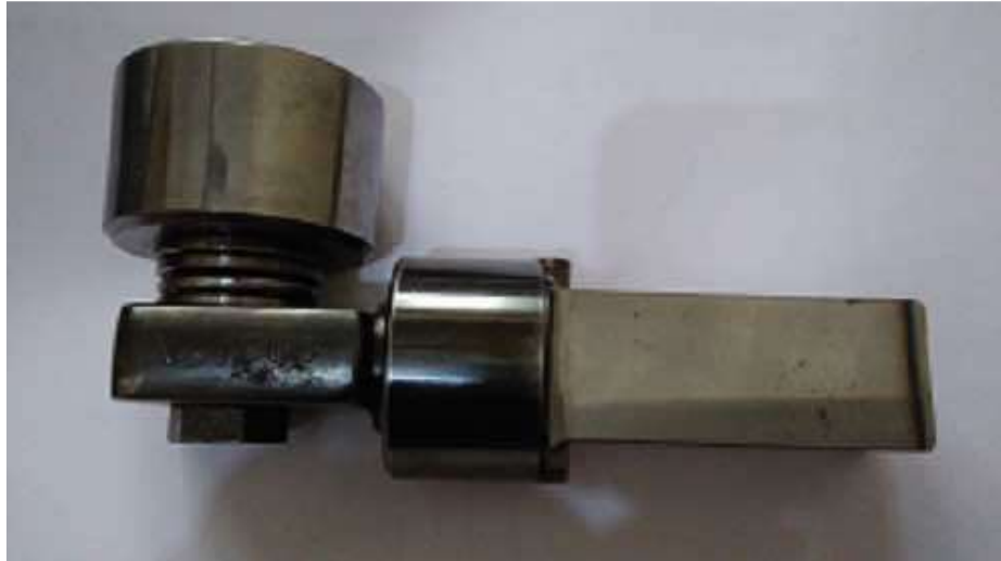
Figure 2.1 Single roller burnishing tool
