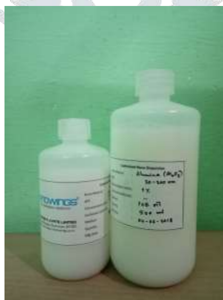
Fig 6: Nano lubricants of Al_2O_3
