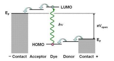
Because of two different materials, an electrostatic force and hence an electric field is set up between the two layers. The conjugated polymers are selected in such a way such that they can create maximum possible electric field and electron-hole pair can be easily broken up by a small energy from external sources (say most of the time solar energy). Electron moves towards electron acceptor conjugated polymer and vacancy of electron (say hole) remains in electron donor conjugated polymer.
