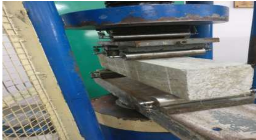
Fig. 4.7 Flexural Test On Beam
