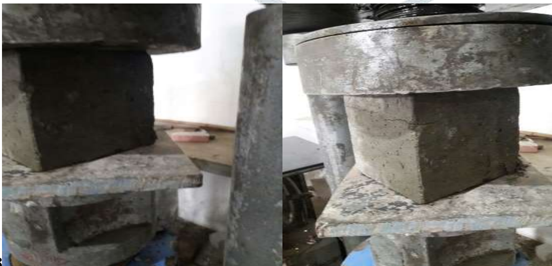
Figure : Concrete cube before and after compression strength test
