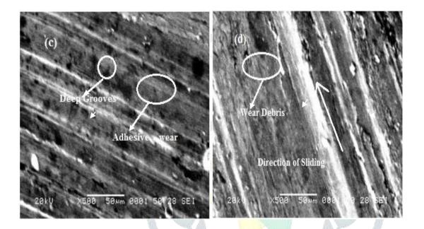
Figure 3 SEM Photographs of the worn surfaces c) 3%SiC 3%B<sub>4</sub>C and d) 7%SiC 3% B<sub>4</sub>C
