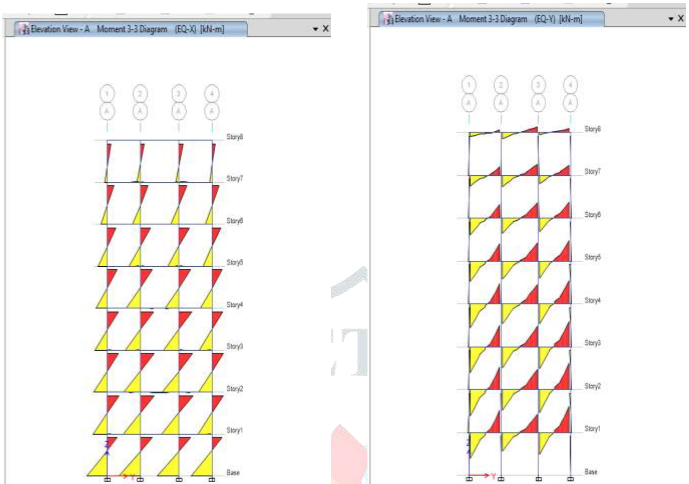
Figure Shows Bending Moment On Each Floor In Both X And Y direction
