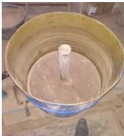
Figure 2 Dry compaction of the layer using a dry standard hammer
