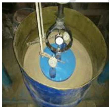
Figure 4 Placing of Proving ring and dial gauge
