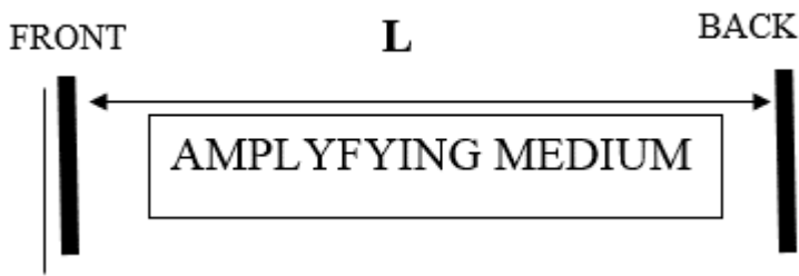
Figure 1.15: Schematic diagram of a basic laser system
