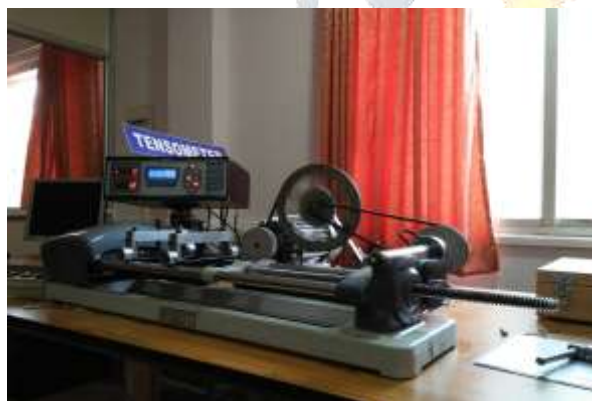
Figure: 2.3.1. Tensometer used for testing tensile
