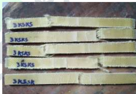
Figure: 2.3.2. Tensile specimen after testing
