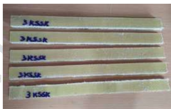
Figure: 2.2.2. Tensile test specimen
