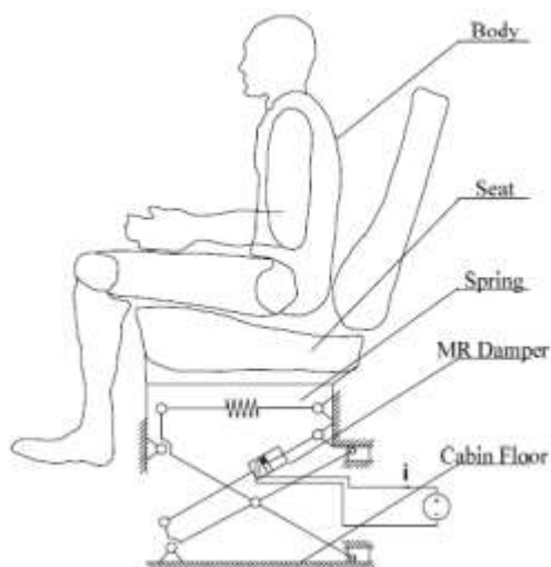
Figure.7. Physical model of semi active seat [17].
