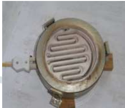
Fig.9 Heater of heat load capacity 1500W
