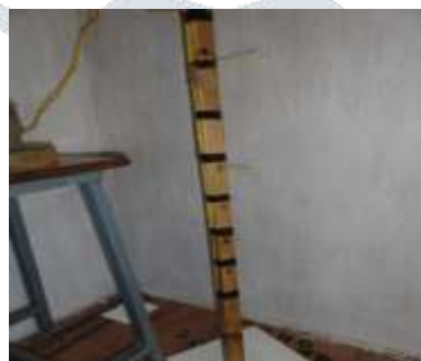
Fig.15 Air temperature measurement with thermocouple
