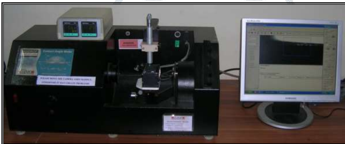
Fig. 2 Contact angle analyzer (Digidrop® Contact angle meter, GBX products, France)
