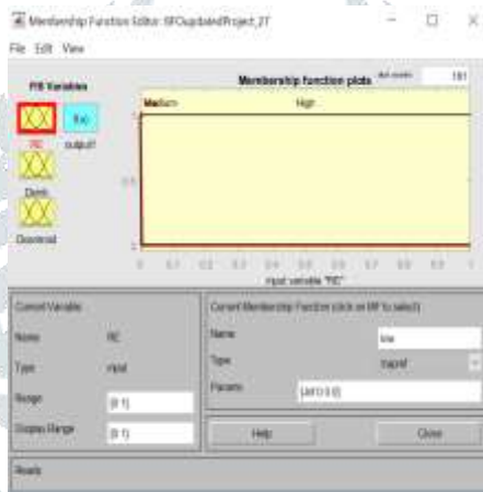
Figure 12 Updated membership function of input RE by using GWO
