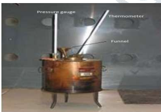
Figure 5 Abel closed-cup flash point apparatus
