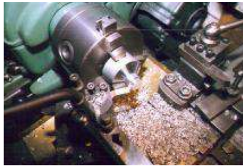
Figure 4.2 Roughing out process
