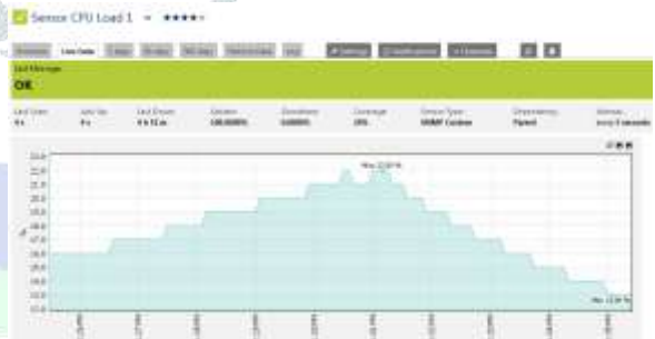
Figure 3.16 - Graph showing decline in CPU Load as IPsec is removed.
