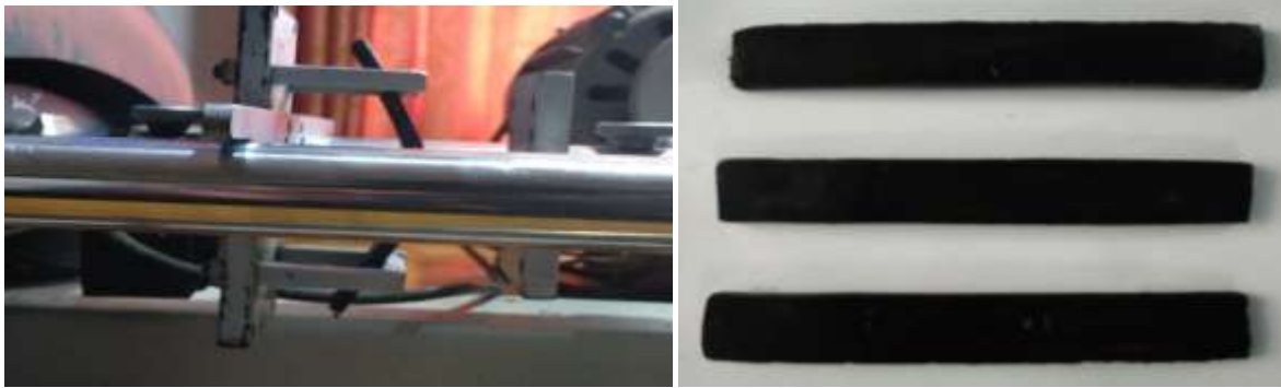
Fig 4: (a) Jaws having the Flexural Specimen (b) Flexural Specimens as per the ASTM standards
