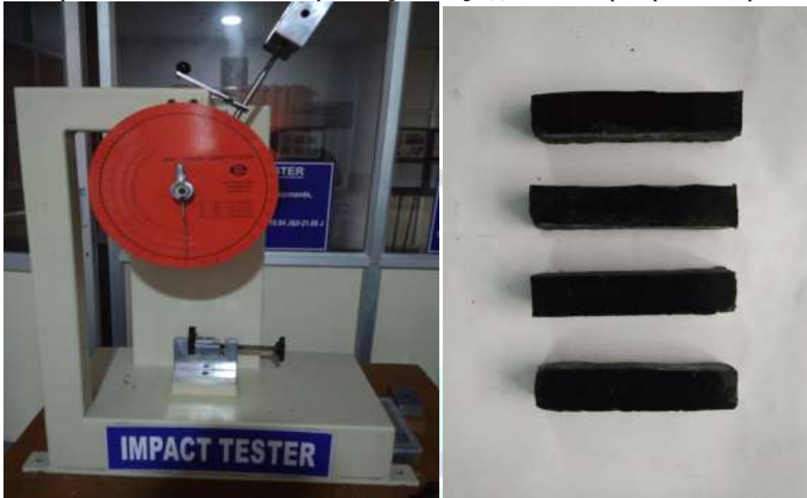
Fig 6: (a) Impact Tester and (b) Impact Specimens as per ASTM standards
