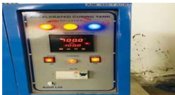
Figure 3 Curing of the Concrete Cubes at a Temperature of 100° C
