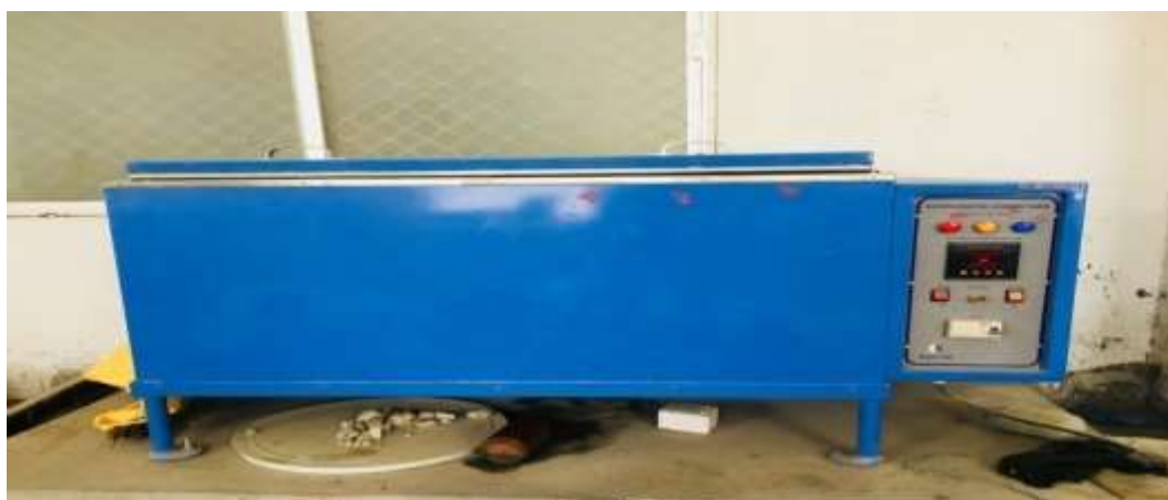
Fig.1. Accelerated Curing Tank
