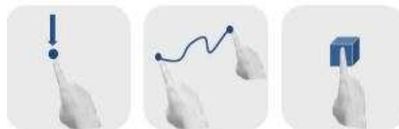
Fig. 1. Spatial program definition through gestures on different levels of industrial robot programming including poses (left), trajectories (center) and tasks (right).
