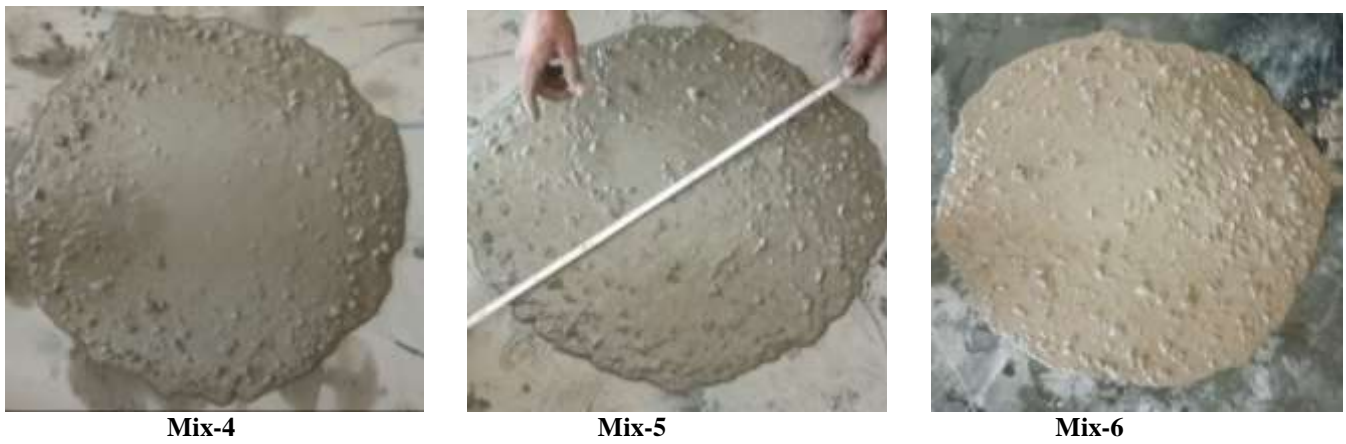
Figure 3: Slump flow for Mix 4, 5 and 6
