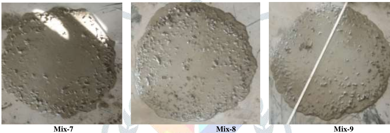
Figure 4: Slump flow for Mix 7, 8 and 9
