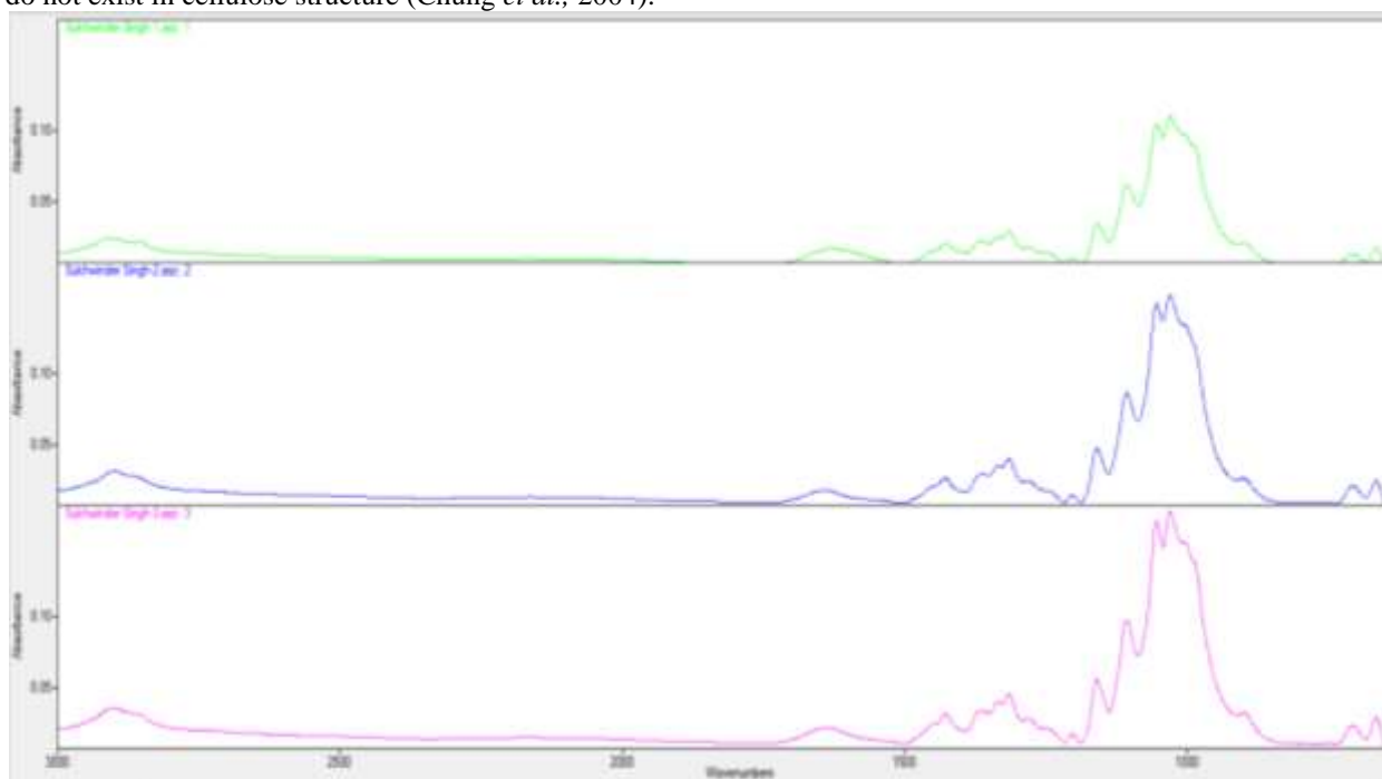
Figure 8 FTIR analysis of cotton fabrics: A) Conventional treatment, B) Enzyme treated (bioscoured), C) Untreated cotton fabric
