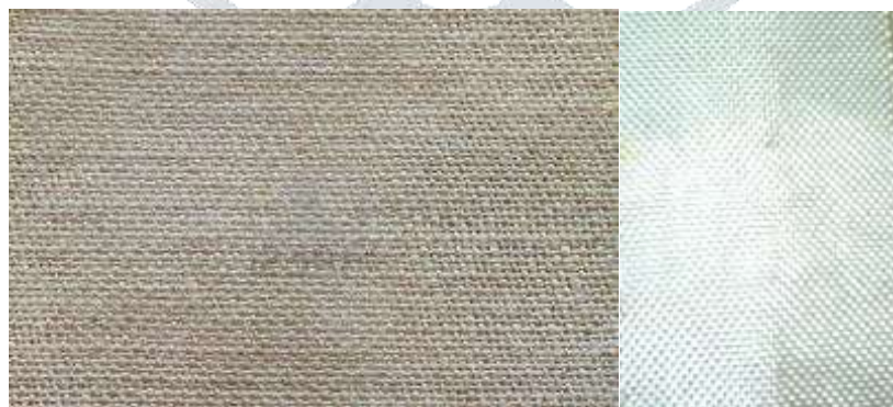
Figure 3 Bidirectional (a) jute fiber and (b) glass fiber
