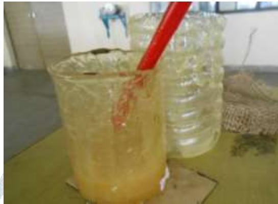
Figure 1 Resin and Hardener mixing
