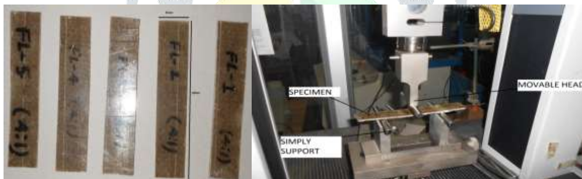
Figure 5 Bending Test Specimen and Testing Setup
