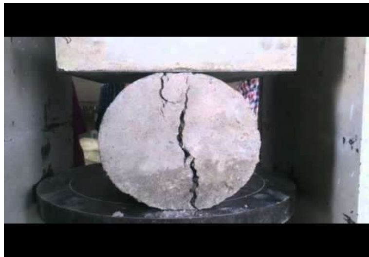
Figure no- 2: Shows the Failure Pattern of Cylinder
