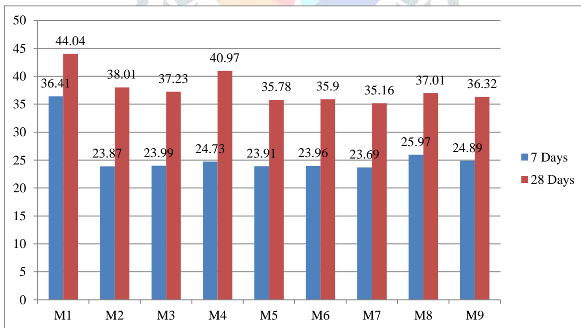
Graph No. 1: Shows the Compression Test Results @ 7 Days and 28 Days
