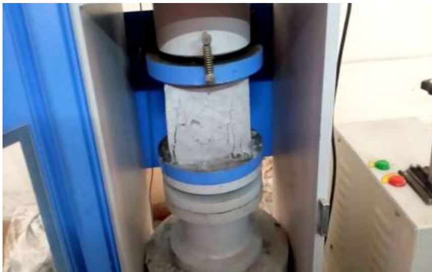
Figure no- 1: Shows the Failure Behavior for Cube
