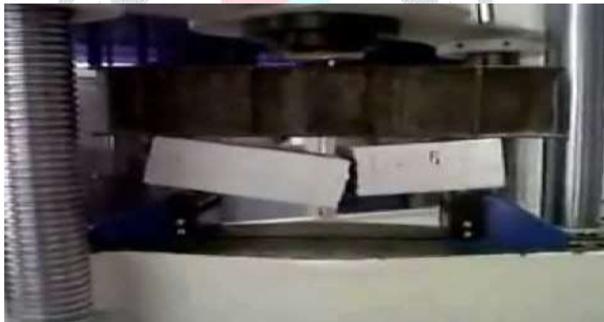
Figure no- 3: Shows the Failure Pattern of Prism
