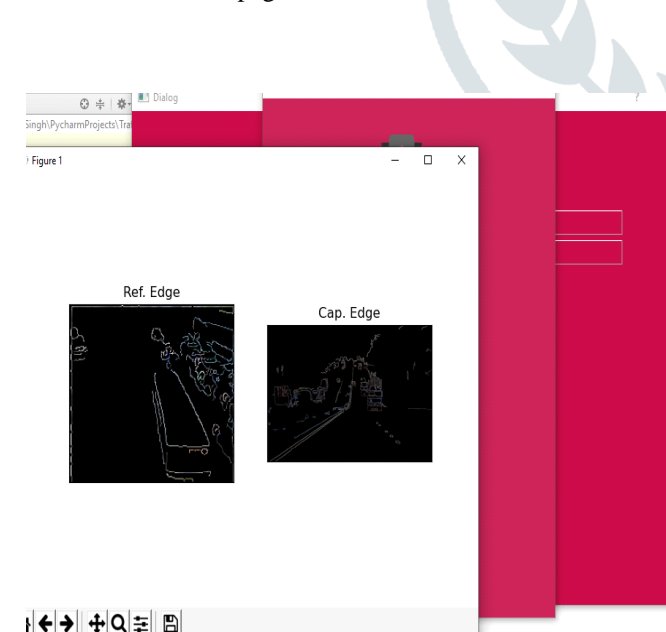
4.8 This is the final output page. After the analysis and detection. It calculates the percentage based on the captured images and reference images. Based on the percentage the traffic signals are adjusted.
