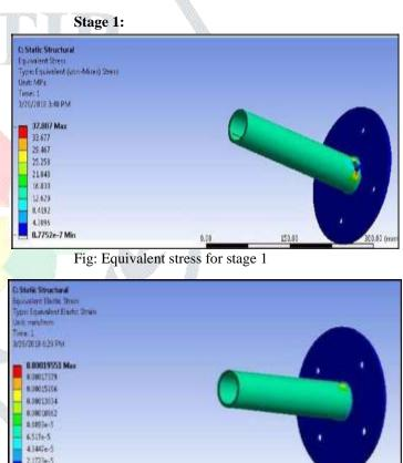
Fig: Equivalent elastic strain for stage 1
