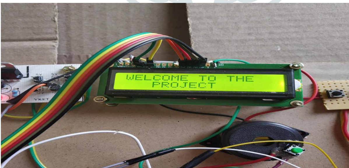
Fig.5.7: After the power supply LCD displays a message "WELCOME TO THE PROJECT"
