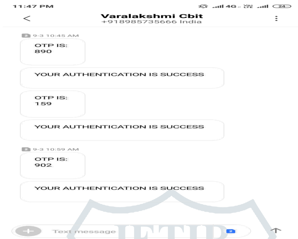
Fig.5.16: OTP is sent to the registered mobile number and if the OTP is correct then the user receives a message “YOUR AUTHENTICATION IS SUCCESS”
