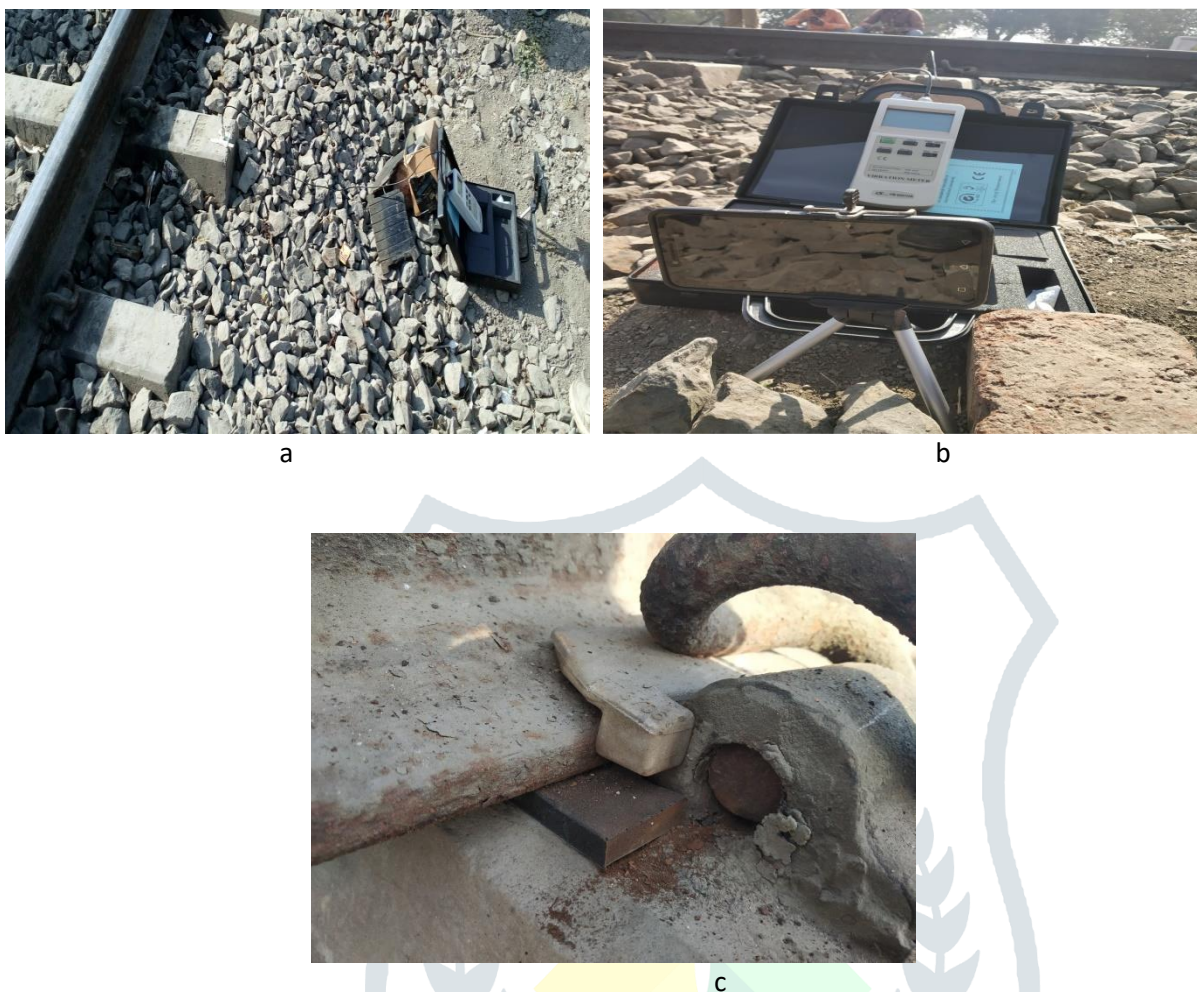
Figure 10: On Field testing a) Probe rested on sleeper b) meter setup prepared c) Sorbothane pads replaced
