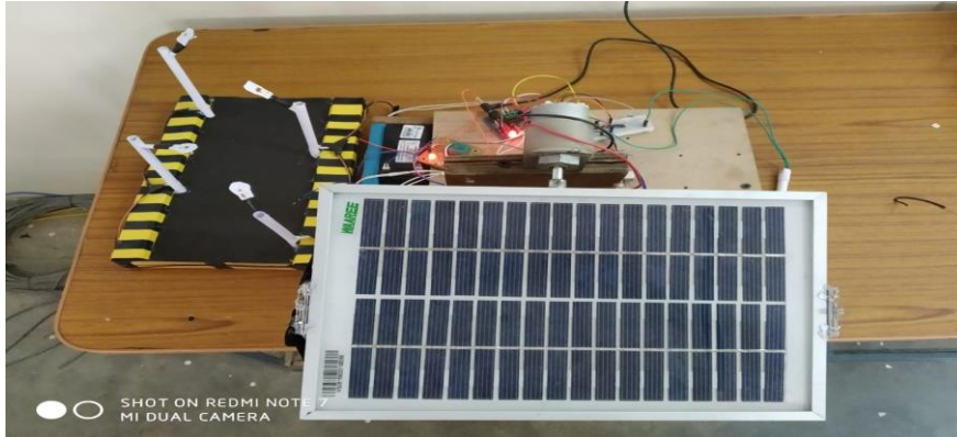
Fig 2: Top View of Automatic Solar Tracker and Auto Intensity Control
