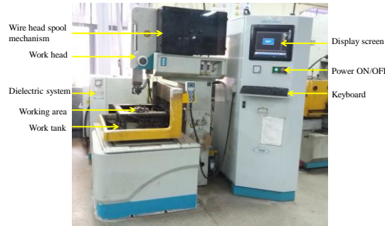
Figure 2 Schematic representation of Wire-EDM
