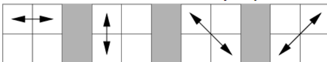
Figure 3.1: Four directions of adjacency as characterized for estimation of the Haralick texture Properties.
