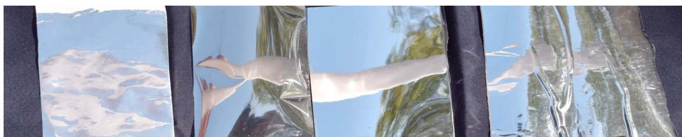
Figure 1: A photo graph of different solar reflective films. From left 1) Aluminium foil tape 2) One-way solar reflective film 3) Mirror wall sticker 4) Vinyl car wrap.
