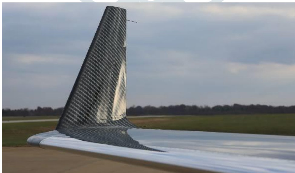
Fig. 1.3. Carbon fibre in aircraft as structure.
