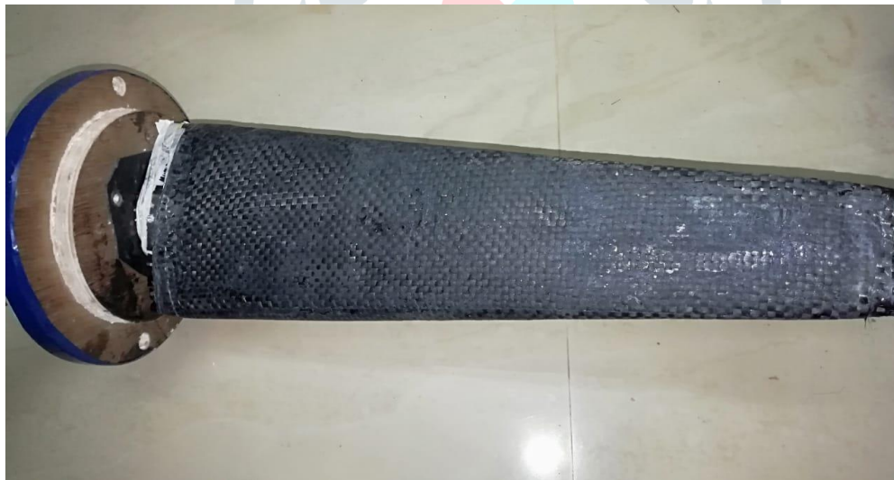
Fig. 2.2 Carbon fibre structural battery.
