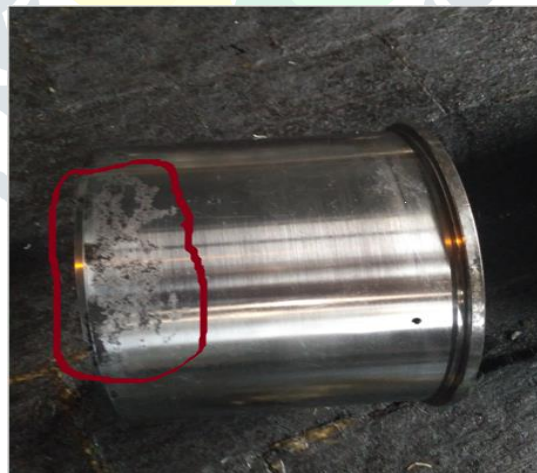
Fig.5: Corrosion on sleeve
