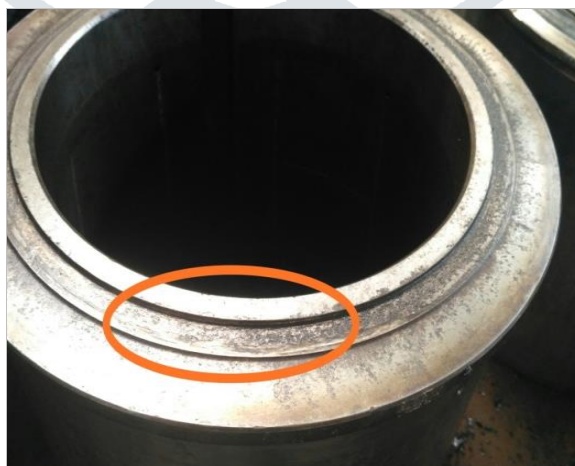
Fig.3: Wear out on sleeve neck
