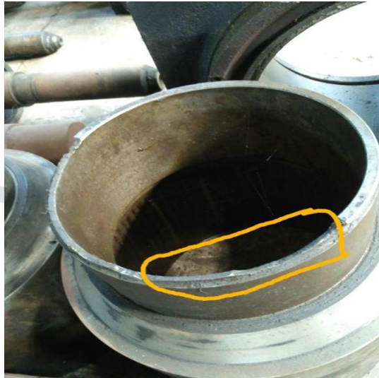
Fig.4: Failure of sleeve at operation side
