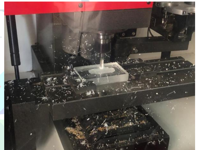
Fig. 4.2 pocketing operation on CNC Machine
