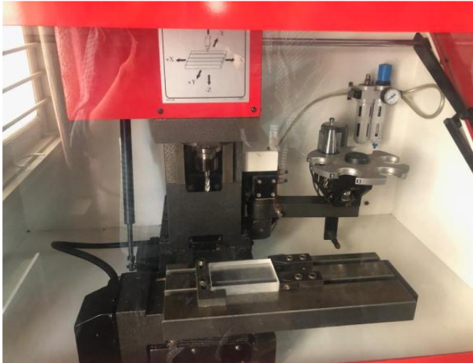
Fig. 4.1 Acrylic Raw material and CNC train simulator
