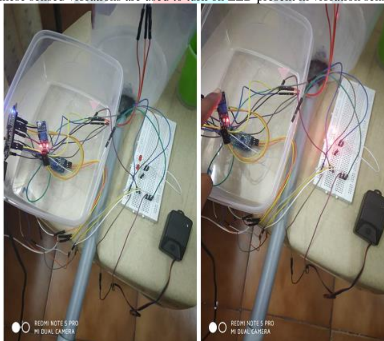
Figure5. (a) Image showing off state of LED due to exposure of LDR to light, (b) shows on state of LED as LDR not exposed to light.
