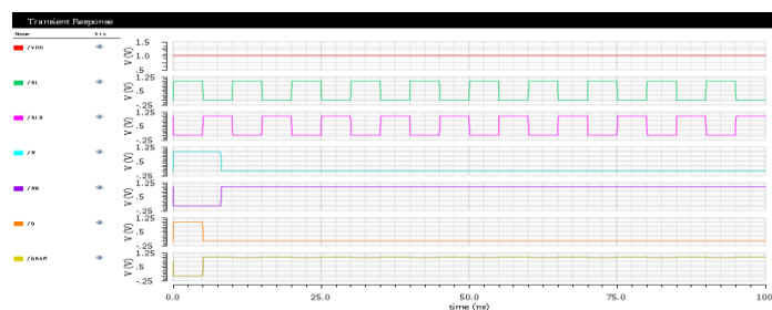
Fig.10. Transient response of the hold operation of proposed 10T SRAM
